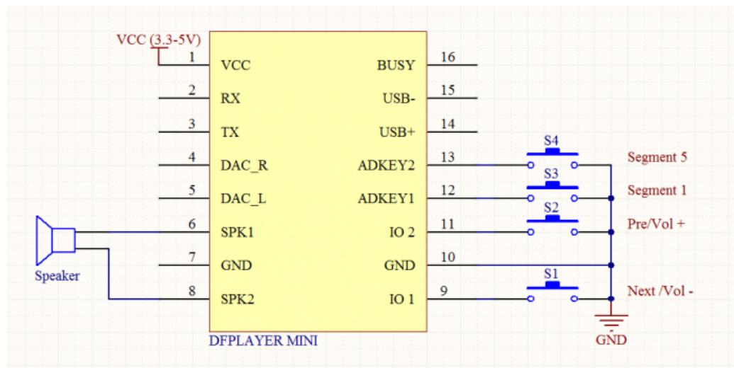
note: short time press means pre/next, and long time press means vol-, vol +
